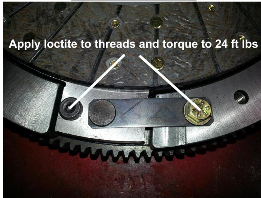
***2. Check the flywheel disc it should spin freely between the flywheel and center plate.***
